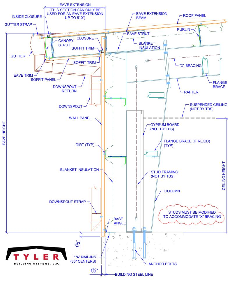
STANDARD SIDEWALL SECTION WITH STUD WALLS
